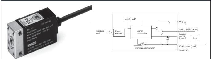
The semi-conductor type pressure sensor and the electronic hybrid circuit are contained in a plastic housing.
