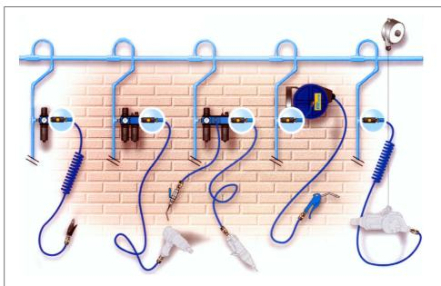
With 6mm orifice you have 50m³/h flow which is suitable for most toolings:
