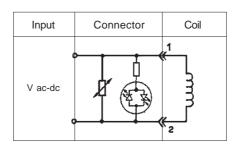
Bipolar LED and VDR to protect supply and switch. (The energy in the coil is limited by the VDR). Voltage: 24 or 230V.
