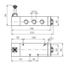
Weight gr. 1152 Minimum working pressure 2,5 bar
