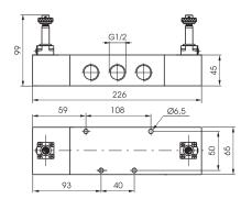
Weight gr. 1744 Minimum working pressure 3 bar
