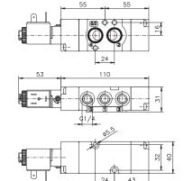
"LT" and "ATEX" Versions are not available with MF coils Weight g. 330 Minimum pilot pressure 2,5 bar
