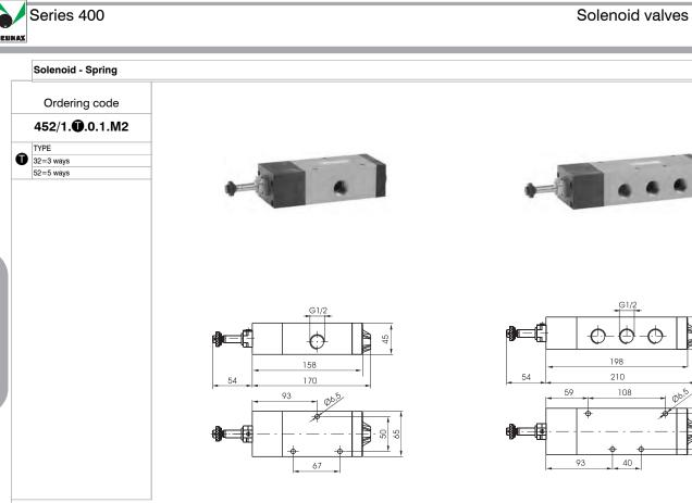
Weight gr. 1330 Minimum working pressure 2,5 bar
