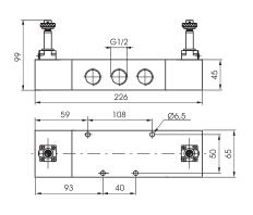
Weight gr. 1474 Minimum working pressure 2 bar
