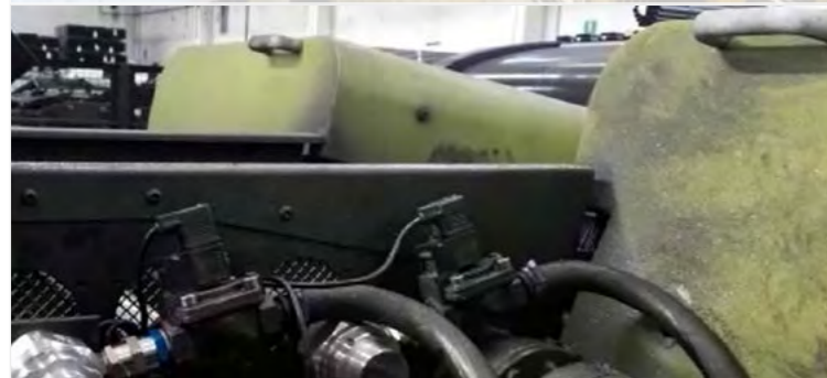
Air amplifiers for profiles' cleaning
