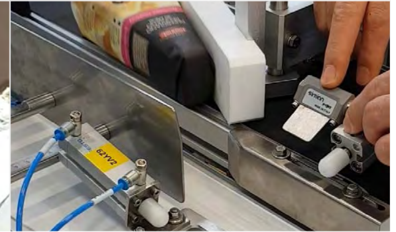
Air knife for defective parts' discard
