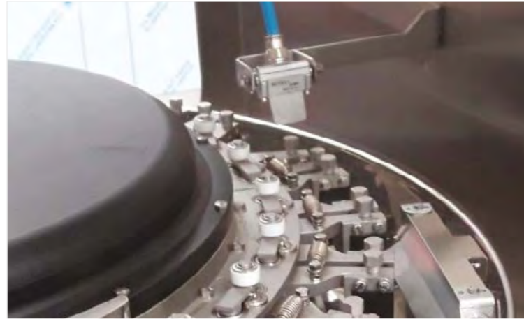
Air knife to dry pharma containers
