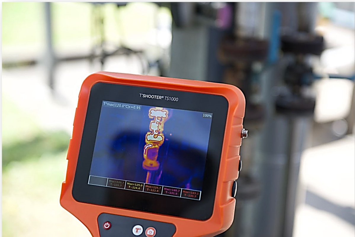
b) – Thermal contour view with Ironbow color
